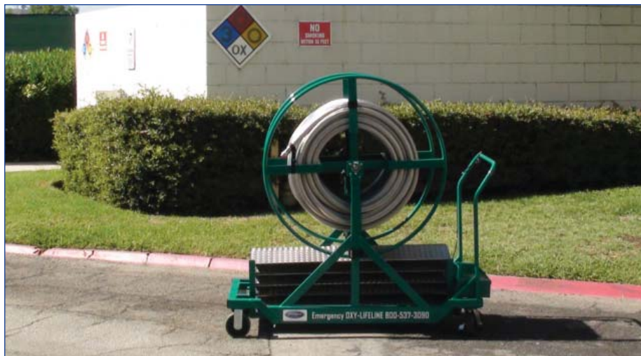
This flexible oxygen tank hose won't break during an earthquake.
