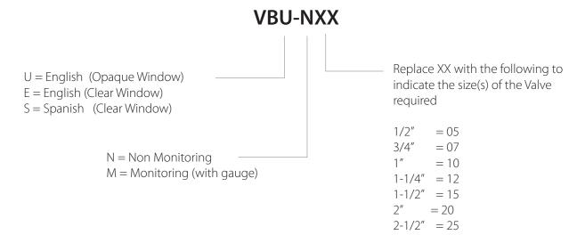
Example: Box with gauge, English (Opaque Window) and a 1-1/2" valve M/N = VBU-M15
