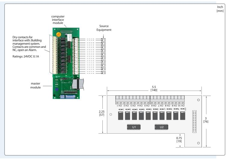
Pull the remote wires from the "Building Management System" into the alarm panel. Make the connection to the terminal blocks located on the side of the module. The wiring is fail-safe normally open, held closed, dry contact to the monitoring equipment.
